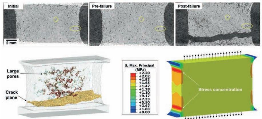
XCT virtual slices showing the middle of an AM manufactured polyamide sample at different stages of loading [top row] together with the 3D view highlighting the larger defects together with the crack plane that are mapped onto the sample prior to failure and a companion FE results showing the stress concentration induced by sample geometry.
