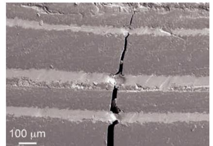
Fracture of an alumina matrix/steel fibre composite fabricated by robocasting
