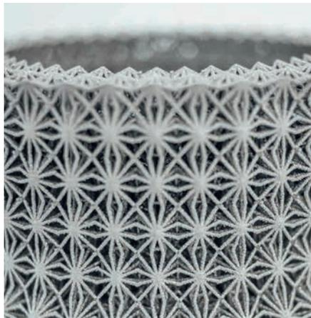
Lattice structure, attractive for a number of applications, such as reducing weight in automotive and aerospace components.
