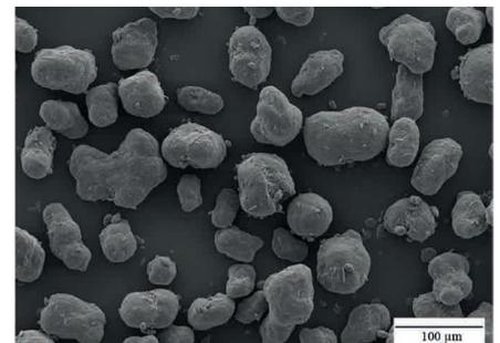
Zhu, Z., et al. [2020] Characterisation and correlation of areal surface texture with processing parameters and porosity of High Speed Sintered parts. *Additive Manufacturing*, **36**, 101402. Micrograph of the virgin PA2200 powders used in this study. Published under Creative Commons CC-BY license. <https://creativecommons.org/licenses/by/4.0/legalcode>.
