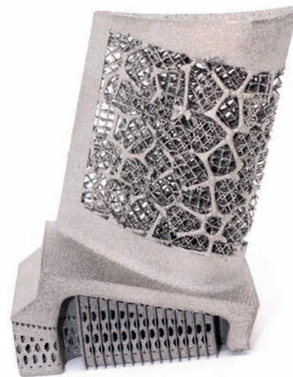
Demonstration artefact showing varying orientations of meso-structures. Pham, M-S., et. al., [2019] Damage-tolerant architected materials inspired by crystal microstructure. *Nature*. **565**, 305-311.
