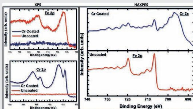
XPS and HAXPES spectrum of Iron and Chromium on uncoated and chromium coated SA508 steel powder. No Iron was detected in XPS spectrum of coated sample whereas HAXPES picked Iron signals on a coated sample.
