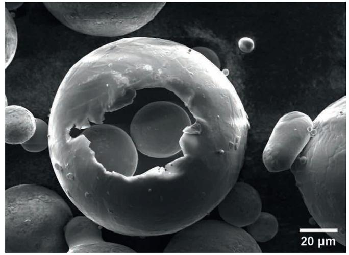
Materials up close runner up Lorna Sinclair. Although usually solid, this Ti-6Al-2Sn-4Zr-2Mo gas atomised powder particle is hollow, and a fractured surface reveals two smaller powder particles hidden inside, likely trapped during atomisation.
