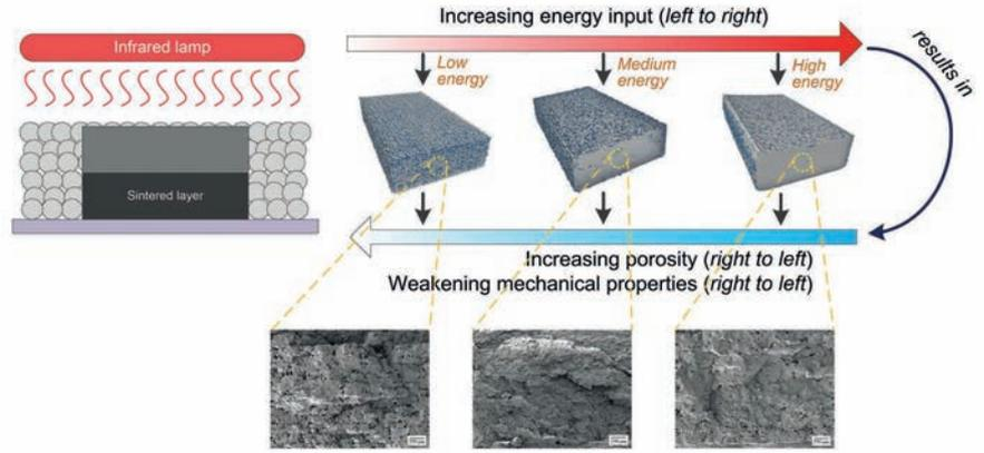
investigation to date relating energy input, pore formation, and the resultant effect on mechanical properties in HSS.
