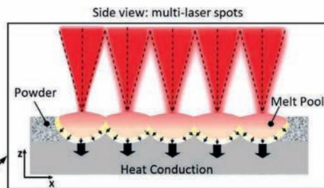
Figure 2 – Individual laser spots and melt pools created on powder bed
