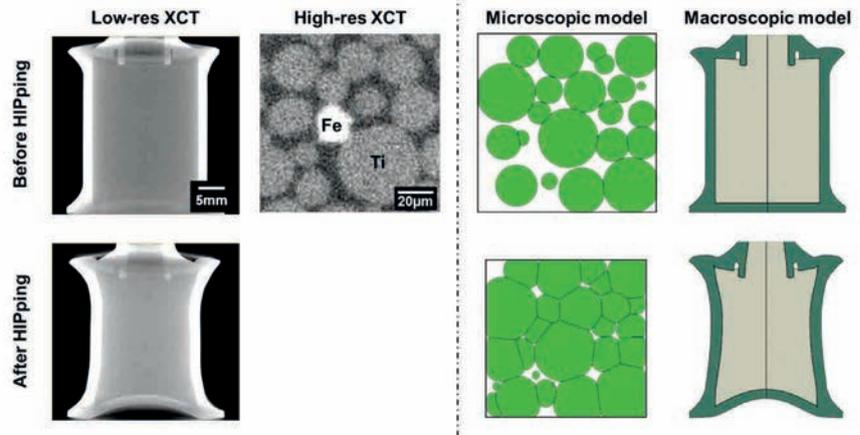
XCT slices [LHS] and microstructurally cognisant models [RHS] showing the sample before and after HIPing on the component [macroscopic] and particle [microscopic] scales.
