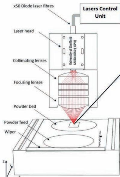
Figure 1 – Diode area melting
