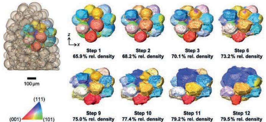
Time-lapse series of sintering steps during densification of the powder body showing a small ROI comprising the nearest neighbour particles, and thus nearest neighbour grains, to the particle containing a fast-growing grain. The location of the ROI with respect to the full sample is illustrated (left). The grains are colored by crystallographic orientation according to inverse pole figure.
