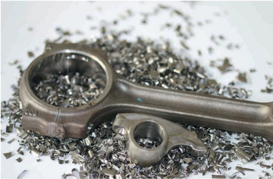
FAST-forge titanium particulate to final component in two steps
