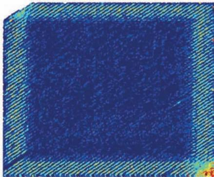
A diagram of the thermal effects of laser history. Heat accumulation can be seen where the laser turns around in the hatch pattern and in the final corner.
