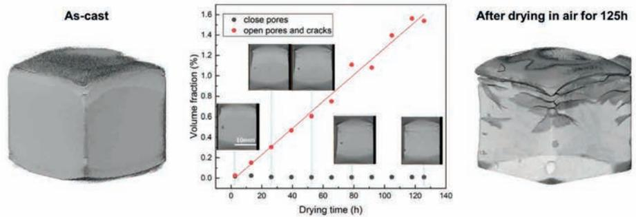
Development of pores/cracks during drying of gel-cast alumina followed by *in-situ* XCT.
