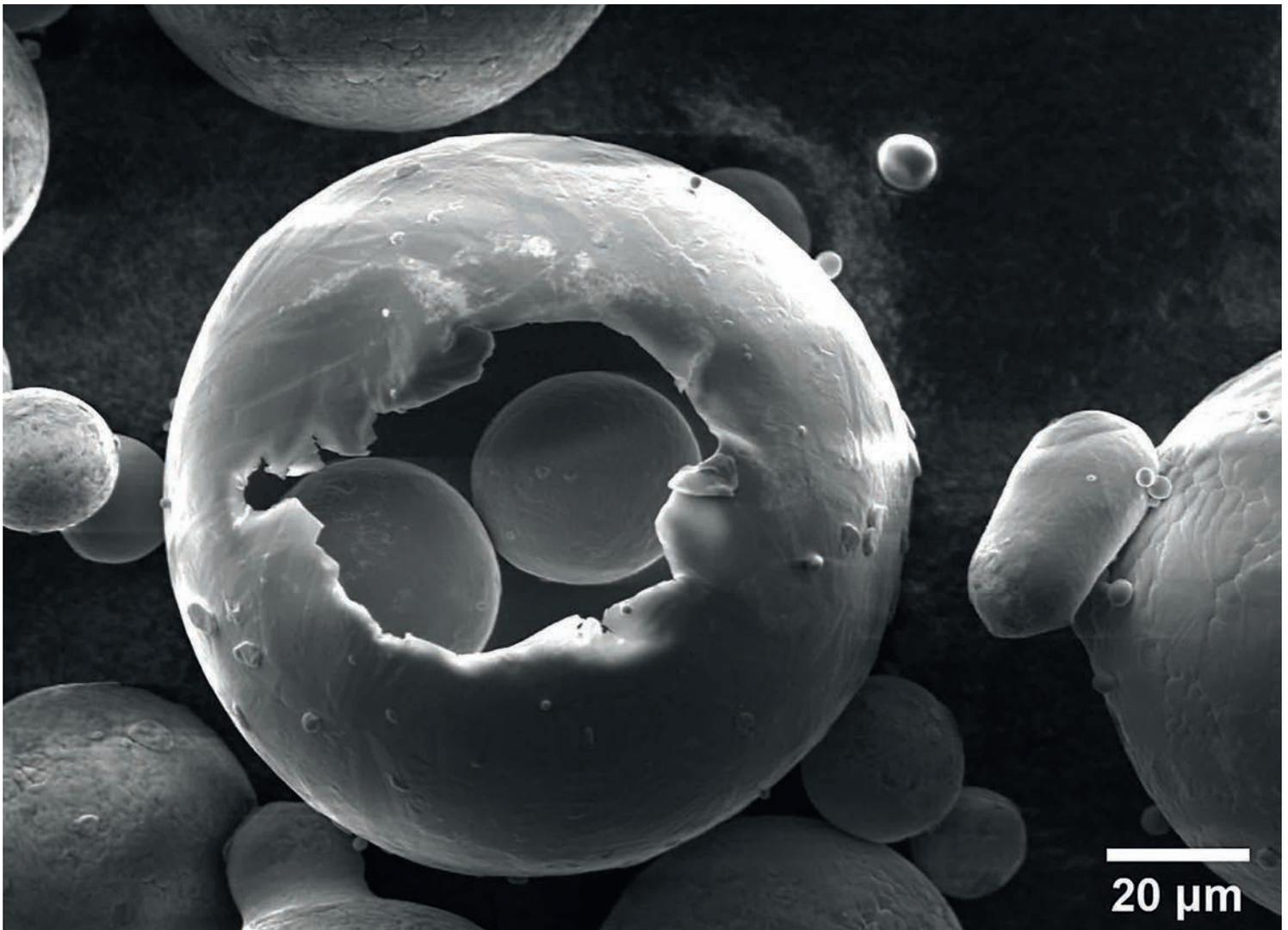
Image above: Scanning electron microscope image of a Ti-6Al-2Sn-4Zr-2Mo gas atomised powder particle by Lorna Sinclair. Although usually solid, this particle is hollow, and a fractured surface reveals two smaller powder particles hidden inside, likely trapped during atomisation. This image was one of the runners up in the MAPP Image Competition, see p18-19 for more information.
