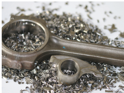
FAST-forge titanium particulate to final component in two steps
