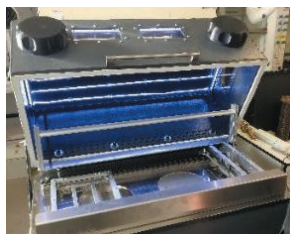
DAM processing chamber and early stage Ti64 sample.
