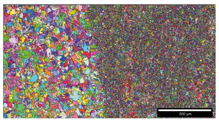
EBSD image of a 2mm x 1mm section of the 0 wt% TiB (left) to 3wt.% TiB (right) interface for a 1400°C 2 hr Ti-6AI-4V sintered sample demonstrating the grain pinning effect of the TiB inclusions
