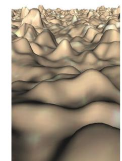
Surface Level from Kieran Nar. A focus variation microscopy obtained surface scan of a polymer laser sintered surface
