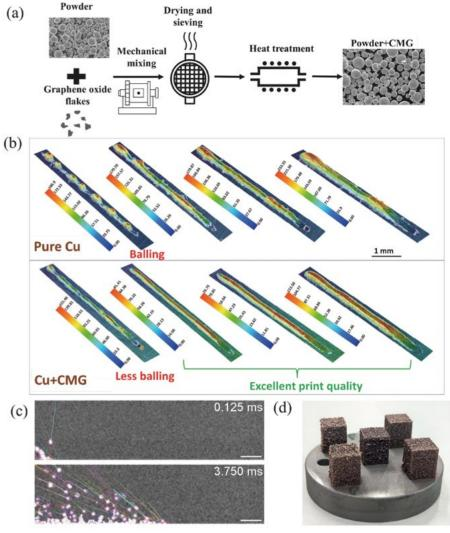
Figure 1. (a) Copper-CMG powder blend preparation. (b) Height map of single tracks for pure copper and Cu+CMG blend showing the improved surface finish and printability with the addition of chemically modified graphene (CMG). [c] Example of in situ process monitoring using synchrotron X-rays where the powder spatter during printing is captured and quantified. [d] Test cubes printed on an industry scale powder bed.
