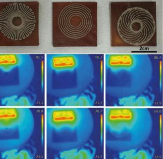
Figure 2. Alignment of hBN platelets during extrusion (inset) combined with direct ink writing enables the printing of materials structures designed to direct heat propagation (from a heat source placed on their side in this example).
