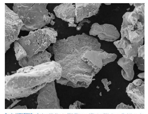
**Cracked HDH Ti64 Powder** from Milo Maguire. SEM, SE image of Titanium 64 hydrogen dihydride powder particles ~100 micron in size. Here instead of atomisation, hydrogen embrittlement has been used to produce the powder. This process allows for brittle fracture of the metal resulting in rough angular morphologies generally detrimental to powder flow. Taken on Hitachi desktop SEM.
