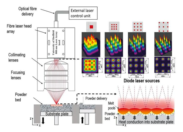
Multi-laser diode area melting - low power short wavelength laser array configurations within a novel 32x32 fibre coupled laser grid, enabling advanced material processing and melt-pool solidification control
