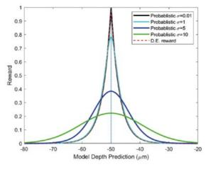
Figure 1. The probabilistic reward function for different levels of prediction uncertainty and a desired target melt pool depth of  $-50\mu m$ . The scaler reward function is shown as a dotted red line.
