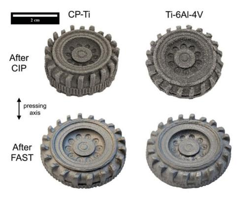
Photographs of CP-Ti and Ti-6AI-4V CIP-FAST parts before and after FAST processing at 980°C for 10 min
