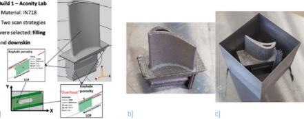
Figure 1. a). Parameter selection using the LPBF diagram for the turbine blade; b). Uncontrolled scan length strategy and c]. Controlled scan length strategy
