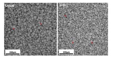
Figure 3 XCT Projection image of SA508 and 316L gas-atomised powders showing internal porosity in the powders (red arrows).
