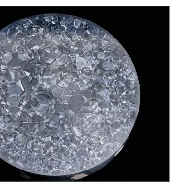
A Look Beneath the Surface from Dennis Premoli. A Ti-64 powder 80mm sample, sintered through FAST, polished and etched (courtesy of Rolls Royce). An attempt at demonstrating the grain growth obtainable through this process and its use is validating new in-process analysis techniques, such as Machining
