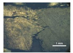
Figure 1. Optical micrograph taken in situ during the fracture of nacre-like graphite showing the action of multiple toughening mechanisms that result in stable crack propagation.
