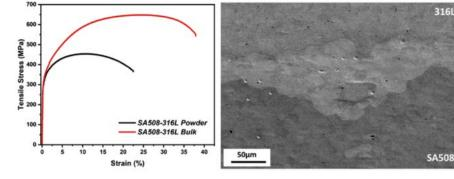
Figure 2 a) Stress-strain curve of the dissimilar joint tested to failure. b) SEM Secondary Electron Image of a FAST joint processed using gas-atomized 316L and SA508 powder at 1100°C with a dwell time of 30 min and 35 MPa pressure.
