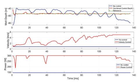
Figure 3. Application of the reinforcement learning, using probabilistic rewards, to the control of the surrogate model.
