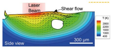
Figure 1. Pore evolution mechanisms in directed energy deposition additive manufacturing revealed with in situ X-ray imaging and multi-physics modelling.
