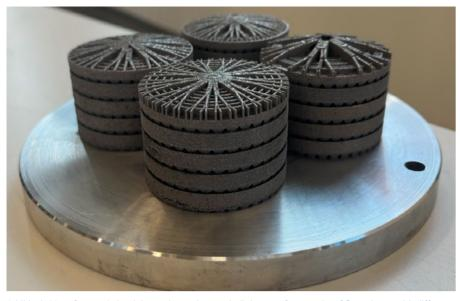
Additively Manufactured aluminium mirrors that are built here as four stacks of five mirrors with different lily-pad lattice designs to reduce the individual component weight. Image courtesy Dr Rob Snell.
