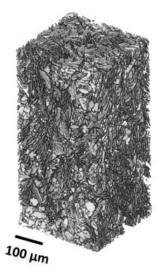
Figure 3. Alignment of microscopic inorganic platelets during processing (in this case hBN platelets in a vitrimer during extrusion) can be analysed using X-ray tomography (in collaboration with the Henry Moseley X-ray Imaging Facility at The University of Manchester]
